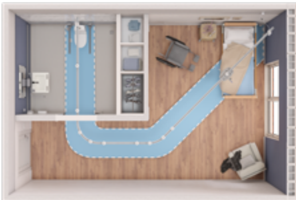
Cost effective. This is a linear layout with multiple curves, crossing the bed, connecting the toilet area. Return to charge (RTC) can be used. When ceiling heights if of concern, a linear tracking layout would maximise stroke (vs X-Y installation). ADL activity could be performed with the walking harness including in bed activities or walking to the bathroom. All typical daily tasks such as bed to wheelchair transfer, transfer to the washroom area can be efficiently performed.
