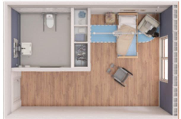
Ceiling mounted. Straight track with curve, providing an out of the way charging area for fixed ceiling lifts.
