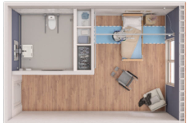
Wall mounted. Linear track, combining wall bracket, side wall posts and T-junction, for fixed or portable ceiling lifts.
