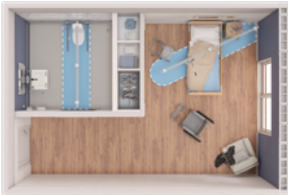
Ceiling mounted. Two separate tracks installed over bed and toilet, (high traffic area for patient handling tasks), possibly a portable lift is best.
