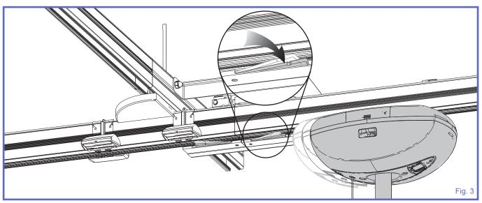
Move the ceiling lift onto the fixed track.
