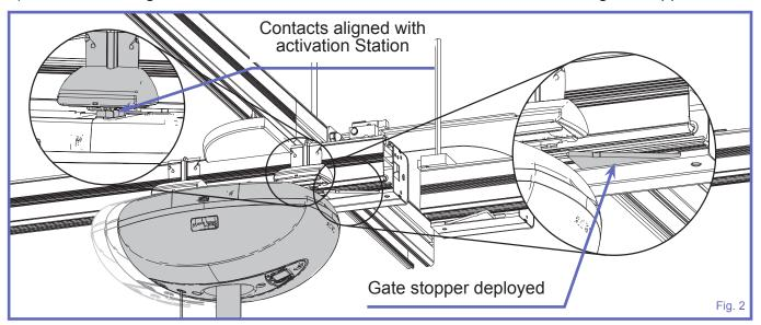
2) Align the mobile track with the fixed track. The gate will clamp both tracks together and the gate stopper will retract allowing the lift to pass through the gate.
