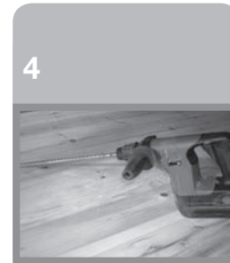
Impact drill with SDS chuck
