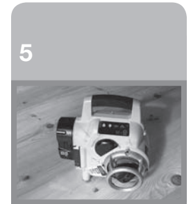
Self-levelling rotating laser
