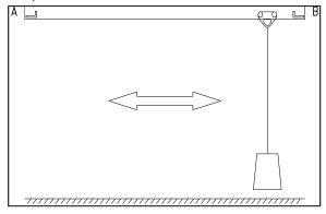
5. Once the weight load test has been completed, lower the weight load to the floor. Remove the trolley by removing the end stopper or the ceiling rail from one end. Remove the trolley from the track. Replace the end stopper or the ceiling rail and tighten with a torque wrench at 15 lb.ft.
