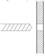
7. Insert the anchors supplied (Part #000.00660) with the installation kit.
